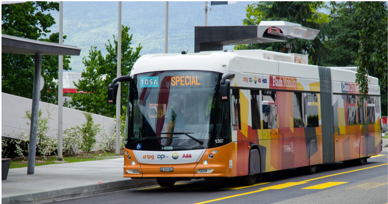
Figure 2.5: TOSA Electric Bus at Charging Station
