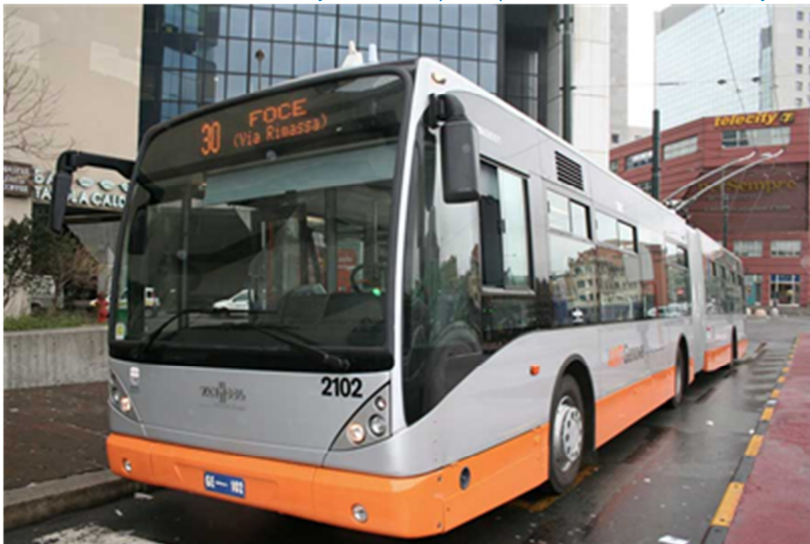
Figure 2.2: Van Hool AG300T Articulated Trolleybus with Super-capacitors and Traction Battery, Genoa, Italy
