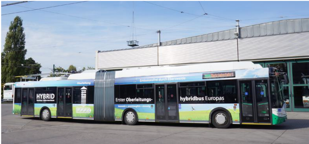
Figure A.2: Solaris Articulated Trolleybus with Traction Battery and Super-capacitors
