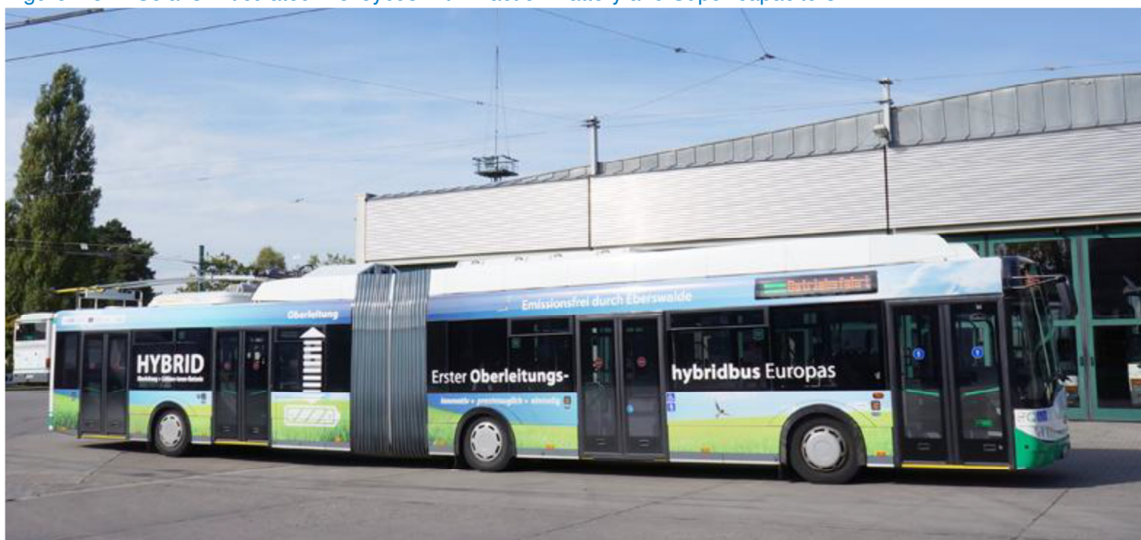
Figure 2.3: Solaris Articulated Trolleybus with Traction Battery and Super-capacitors
